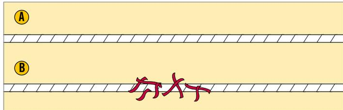
The LOEPFE method using optical measurement detects and removes the faulty or disturbing yarn. Systems measuring the mass can hardly detect this difference.
