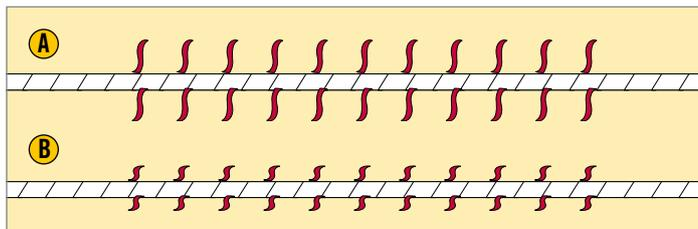
The LOEPFE method using optical measurement detects and removes the faulty or disturbing yarn. Systems measuring the mass hardly detect the difference because the mass difference is too low.
