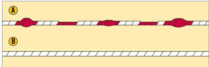
**LOEPFE uses optical measurement to detect and remove the disturbing yarn.** Systems measuring the mass can hardly detect the difference.
