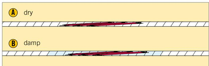
**The LOEPFE method using optical measurement is not influenced negatively by deviating measured values.** Systems measuring the mass identify a supposed yarn difference.
