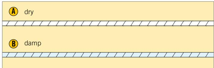
**The LOEPFE method using optical measurement is not influenced negatively by deviating measured values caused by humidity changes.** Systems measuring the mass identify a supposed yarn difference.
