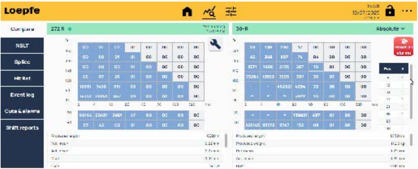
Comparison of one spinning position with the whole machine
